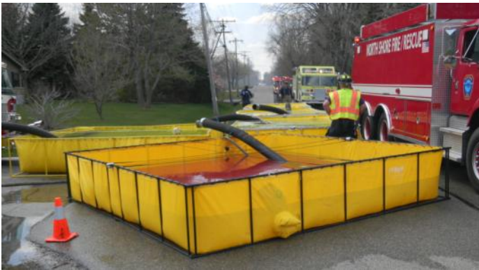
Top: an engine, drawing from a Port-a-Tank, supplied several hand lines. The truck behind it was supplied by additional Port-a-Tanks. Left: a block away, 5 Port-a-Tanks were supplied by the tenders. Below: the block-long hose layout. (Photos by Gary Schmidt)
