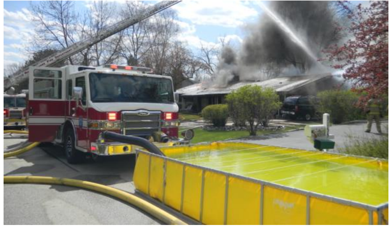
Top: an engine, drawing from a Port-a-Tank, supplied several hand lines. The truck behind it was supplied by additional Port-a-Tanks. Left: a block away, 5 Port-a-Tanks were supplied by the tenders. Below: the block-long hose layout. (Photos by Gary Schmidt)
