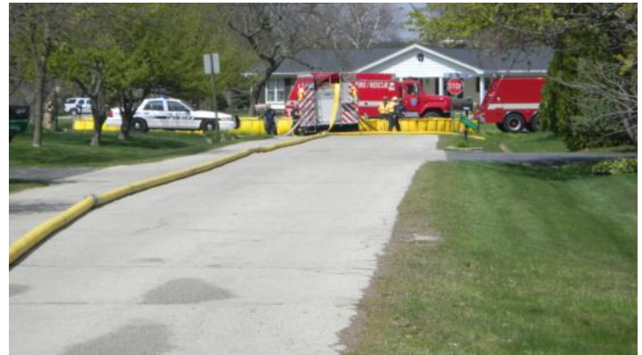
Top: an engine, drawing from a Port-a-Tank, supplied several hand lines. The truck behind it was supplied by additional Port-a-Tanks. Left: a block away, 5 Port-a-Tanks were supplied by the tenders. Below: the block-long hose layout. (Photos by Gary Schmidt)
