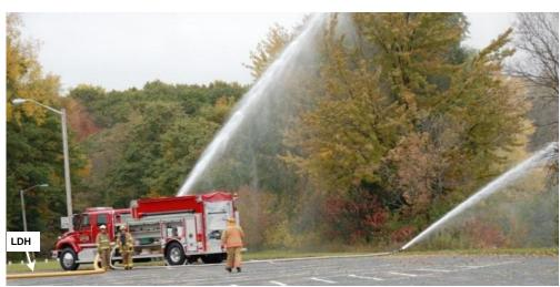
At left, shown is the end result: the ability to use pressurized hose lines for fire attack.
