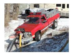
The pickup with the front mount pump is used to fill tenders or as a relay truck. It set up by a river just down the street from the fire scene and was used to relay water to our attack engine as a supplement to the water supply we had set up. It is a very handy truck to have in a rural area!!
